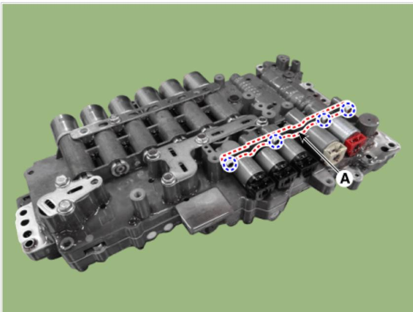
8. Remove the R position solenoid valve (A).
