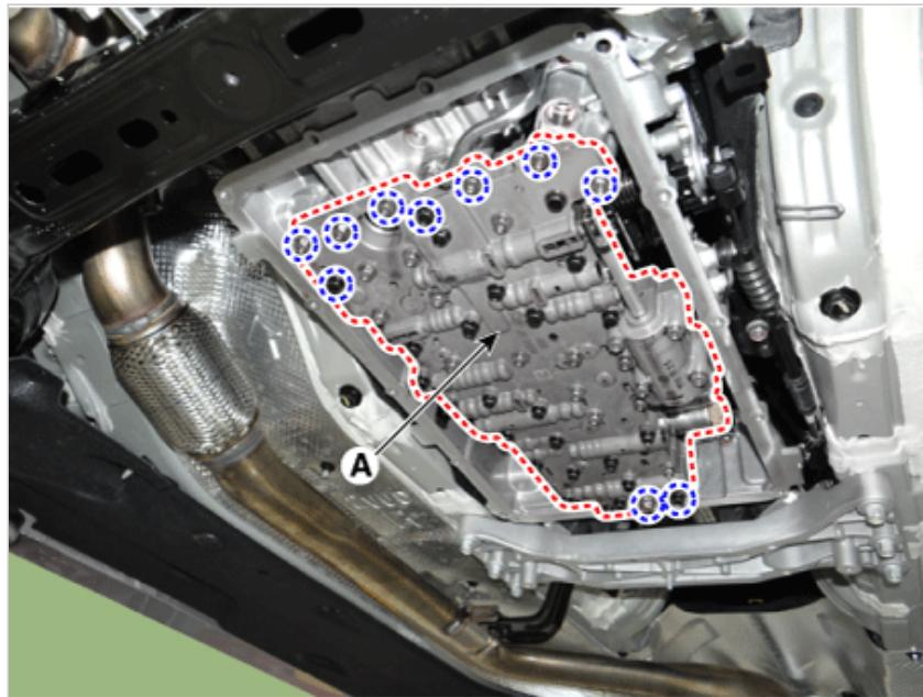
6. Remove the E-module (A) after loosening the bolts.
